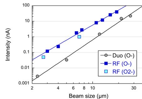
**Fig. 1.** Intensity of primary ions versus beam sizes of RF Plasma source. DP source data are from [5,8-9].
