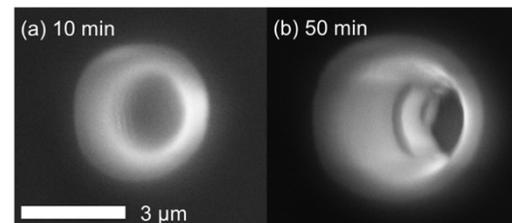
**Fig. 2.** SEM images of SIMS pits made by  $50$  pA  $\text{O}_2^-$  primary ion beam on labradorite standard. (a) 10 min sputtering for alignment. (b) After 50 min of Mg isotope analyses with  $1$   $\mu\text{m}$  rastering.
