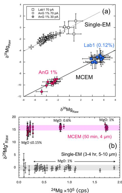
**Fig. 3.** Mg isotope analyses of plagioclase standards using MCEMs without correcting for relative gains of detectors. Single collector axial EM analyses from [3, 8] are shown for comparison.
