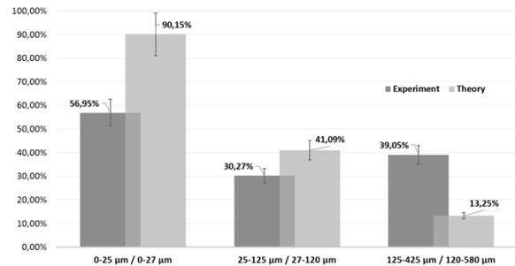
Figure 2. Theoretical and experimental carbon survival in particles of different size.
