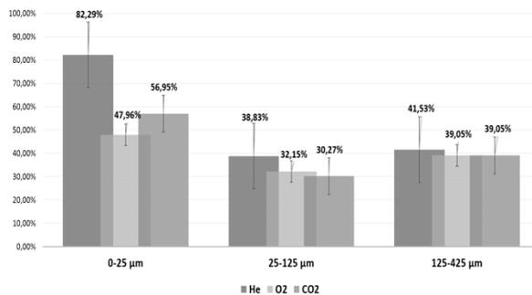
Figure 1. Surviving carbon percentage using different carrier gases.
