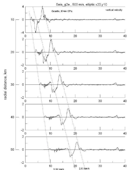
Fig. 1. A classic wave surface pattern in a hard rock target for a low velocity ( $0.5 \text{ km s}^{-1}$ ,  $D_{\text{proj}} \sim 3 \text{ km}$ ) impact. The model reproduces the longitudinal and Rayleigh wave ( $5.5$  and  $2.9 \text{ km s}^{-1}$  correspondingly). Time is in seconds.
