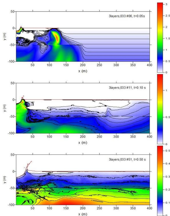
Fig. 3. Three time frames for the 1 kms<sup>-1</sup> impact ( $D_{proj}=10$  m, lunar gravity) into 3-layers target: 10 m “sand”, and 50 m “tuff” over a hard rock basement. Zero pressure (“spalled”) near surface zone reaches ~8 crater radii.
