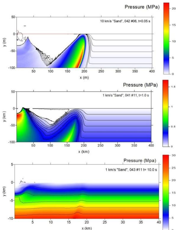
Fig. 2. “Spallation” near-surface zone in modeling of 10 kms<sup>-1</sup> (top panel) and 1 kms<sup>-1</sup> (middle and bottom panels) impacts into an uniform soft (“sand”) target. Only the large natural lithostatic pressure (bottom panel, projectile diameter 1 km) suppresses the origin of zero-pressure (“spalled”) zone behind the shock wave sliding along the free surface.
