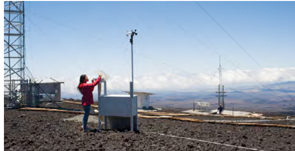
Fig. 1. Filter exchange in the high-volume air sampler at Mauna Loa Observatory.
