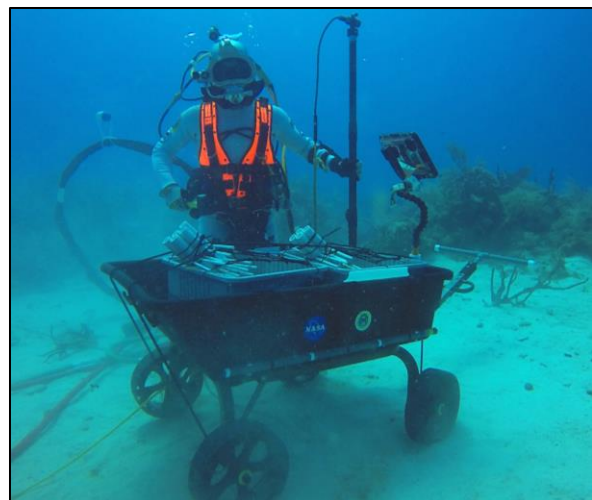
Figure 1: The METS including camera and tablet mounts and Modules loaded inside the cart.
