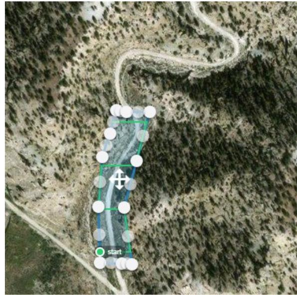
**Fig. 2.** Google-Earth view of the region of study in Utah. The image roughly covers a 500x500 m area. A 3 minute flight at 100 m elevation would cover an area  $\sim 200 \times 50$  m in adequate overlap for high resolution mosaics and DTM construction. Image credit: Drone Deploy and Google Earth.
