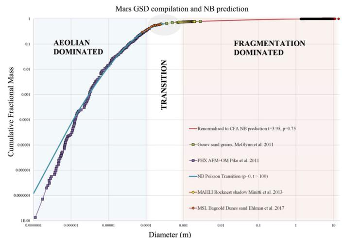
Figure 1: Cumulative fractional mass versus diameter distribution over 8 orders of magnitude and NB fragmentation models. Sand size particles are from Spirit and Gusev landing sites [3,4,7], particles 0.1 mm are from Phoenix [18], and rock distributions are from orbital images of the InSight landing site [10]. Note the transition in the fragmentation curves between impact dominated processes above 0.2–0.5 mm and eolian dominated processes below.
