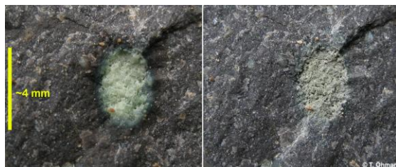
Fig. 2. Kärnäite includes an unknown mineral that changes its color from green to grey within minutes of being exposed.
