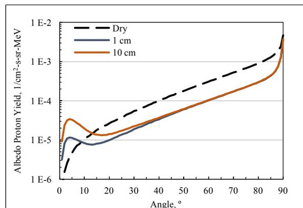
**Figure 1.** A comparison of the GCR induced albedo proton emission spectra as a function of off-zenith emission angle for dry regolith, 1 cm water, and 10 cm water.
