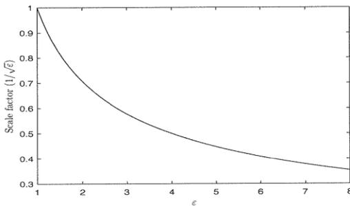
**Figure 2:** Sensitivity of retrieved reflector distance to permittivity is described by the scale factor  $1/\sqrt{\epsilon}$ .
