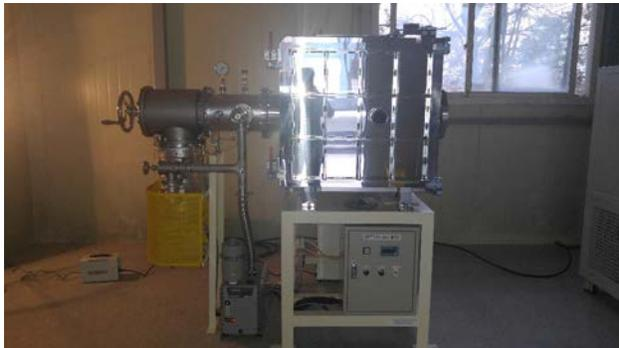
Figure 1. Contaminant Control Chamber for testing contaminant trapping.
