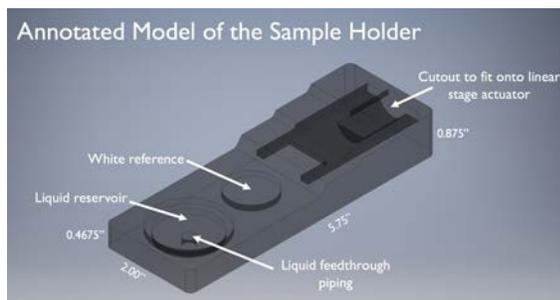
Figure 4. Current sample holder, which is being improved.
