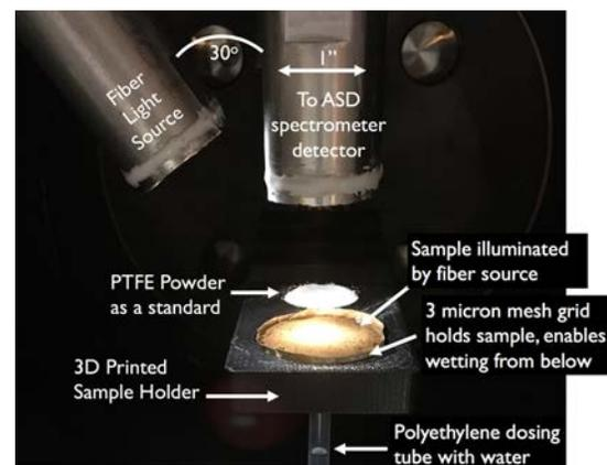
Figure 2. A sample and standard in the sample holder in the MARS chamber while illuminated by fiber optic light during spectral collection. We are modifying the sample holder to be ~ 6" long and capable of exploring downslope transport of water and mass movement.
