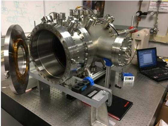
Figure 1. The Mars Analog Reflectance Spectroscopy (MARS) chamber. Achieve Mars pressure, N<sub>2</sub> or CO<sub>2</sub> background, Mars chamber, and equipped with an ASD FieldSpec Pro for spectral acquisition from 0.4 to 2.4 μm.
