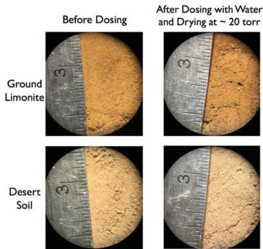
Figure 3. The surface of the sample is roughened as water sublimates from sample under Mars conditions. This roughness increases shadowing that could explain the darkening of RSLs even when moisture is no longer present.
