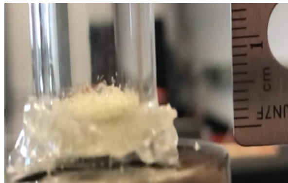
Figure 1: Shaking tube experiment at 40 Hz. Peak grain height <1 cm.
