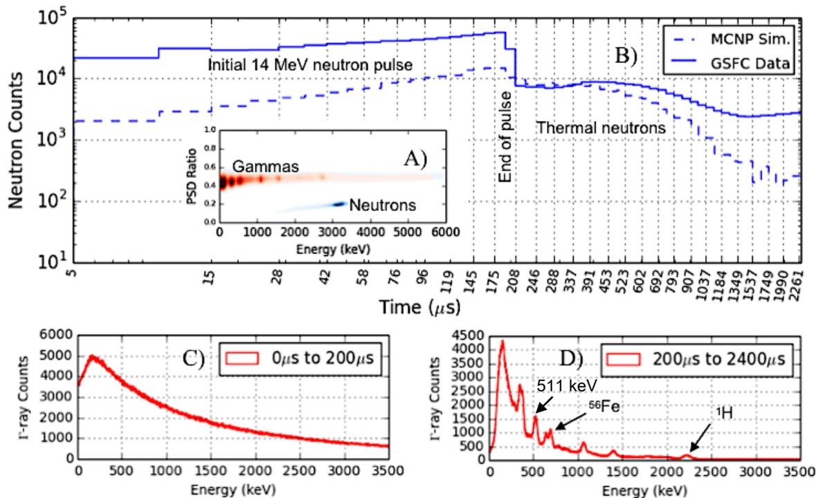
Figure 2: Preliminary results for an hour long PNG experiment with  $10^7$  neutrons per second pulsed at 250 Hz, with 2 inch thick polyethylene located under 20 cm of basalt: A) the resulting PSD plot (0 to 2400  $\mu$ s), B) neutron die-away plot, c) gamma-ray plot during the pulse (0 - 200  $\mu$ s), and D) gamma-ray plot after the pulse (200 - 2400  $\mu$ s).
