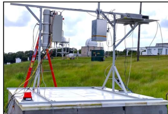
Figure 1: Outdoor test set-up at GSFC GGAO showing the basalt monument, poly blocks, the PNG, SINGR detector, and electronics.
