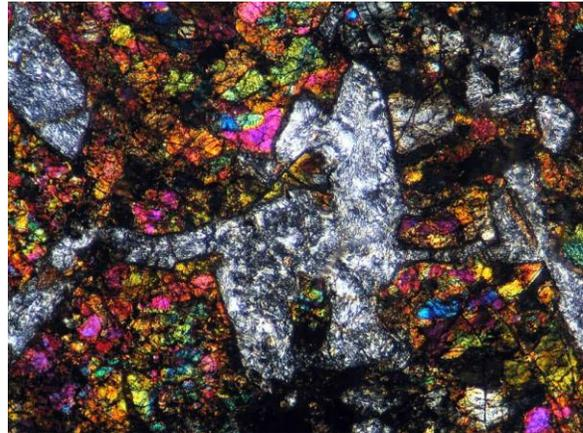
**Figure 1.** Cross-polarized thin section image of NWA 2824 showing spherulitic plagioclase (gray) and recrystallized, polygonal-mosaic pyroxene (colors).
