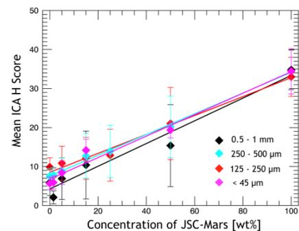
Figure 1: Hydrogen ICA scores for mechanical mixtures between JSC-1 lunar simulant and JSC-1 martian simulant for 4 ranges of grain sizes. Error bars represent the standard deviation.
