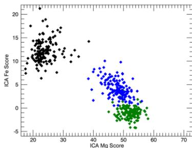
Figure 3: ICA Mg scores as a function of ICA Fe scores for pure JSC-1 lunar simulant grains 125-250  $\mu\text{m}$  (black dots), pure magnesium sulfate (green dots) and grains JSC-1 lunar simulant grains (125-250  $\mu\text{m}$ ) with 15 wt%  $\text{MgSO}_4$  surface coatings (blue dots).
