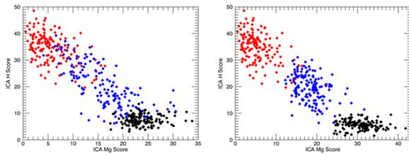
Figure 2: ICA Mg scores as a function of ICA H scores for pure JSC-1 lunar simulant (black dots), pure JSC-1 martian simulant (red dots) and two mechanical mixtures of these products (50 wt% of alteration compound) with grain sizes: 125-250  $\mu\text{m}$  (left) and < 45  $\mu\text{m}$  (right).
