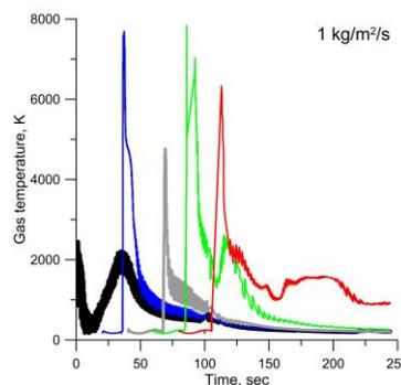
**Fig. 2.** Temperature around 5 representative 1-mm-sized particles that are 20 s apart within ejecta arriving over 100 s. Compared to Fig. 1, the maximum temperatures are much higher (up to 10000 K, but the total duration is shorter (~10 s). Some particles are entrained within a rising flow of hot gases and are subjected to the second pulse of heating (see red and green curves and also Fig. 3).
