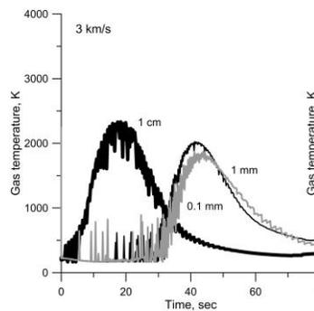
**Fig. 1.** Gas temperature during the re-entry of 0.1 mm-1cm particles at 3 km/s. The total mass is 100 kg/m<sup>2</sup>, i.e., ejecta deposits are 4-cm-thick. All particles arrive at the top of the upper atmosphere simultaneously.
