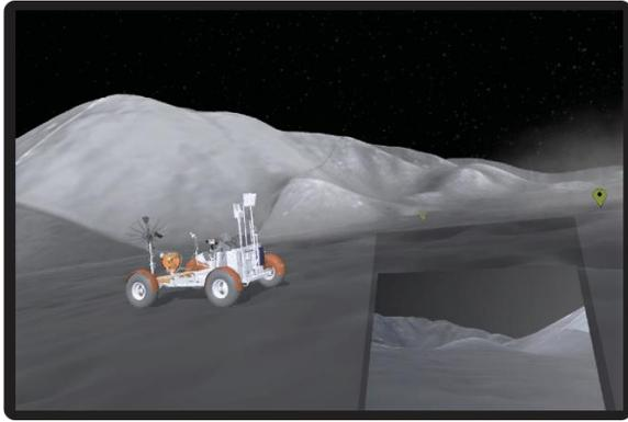
**Figure 3:** HUD shows the view from the lunar rover camera as it navigates autonomously to waypoints
