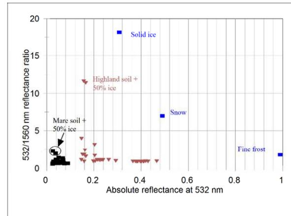
**Figure 1.** 532/1560 nm reflectance ratio versus absolute reflectance at 532 nm for highland and mare simulants as described above.
