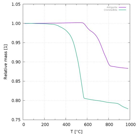
**Figure 1** - Mass loss curve for Antigorite and Cronstedtite under inert gas flow.
