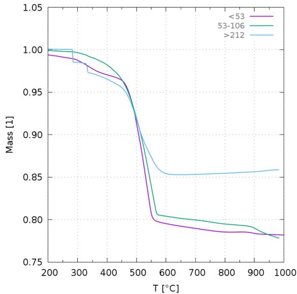
**Figure 2** - Comparison of dehydration process for various grain sizes of Cronstedtite.
