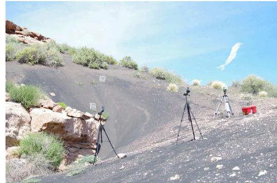
Figure 2: Setup on a falling dune at Grand Falls. Two high resolution video cameras, two calibration targets and a Terrestrial Laser Scanner are visible.
