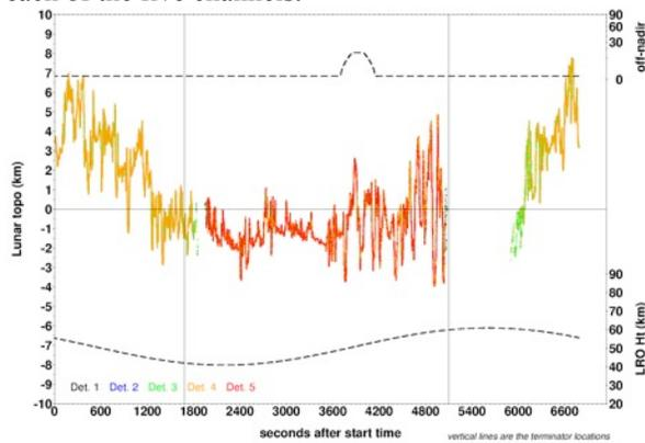
Figure 1. Altimetric profile of orbit 5709 (2010/09/20).
