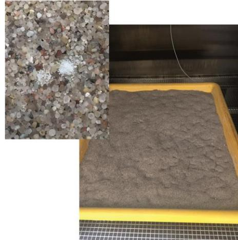
Fig.6. Experiment no 4. Dry sand 1 mm with a dry carbon dioxide underground layer in granular form. Quantity of CO<sub>2</sub> granules used - 6 kg. This Fig.6 refers to Fig.7.
