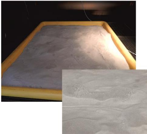
Fig.4. Experiment no 3. Dry sand (0.3-0.6 mm) with brine layer underground (150g NaCl/ l). (amount of brine used in the form of ice:4.5 l). This Fig.4 refers to Fig.5.
