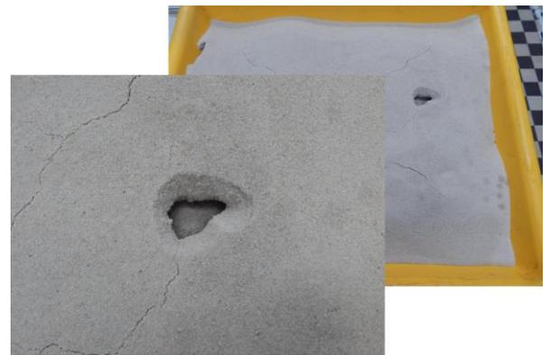
Fig1. Experiment no 1. Dry sand (0.3-0.6 mm) with ice layer H<sub>2</sub>O underground (amount of water used to produce ice: 2.5 l. This Fig.1 refers to Fig.3
