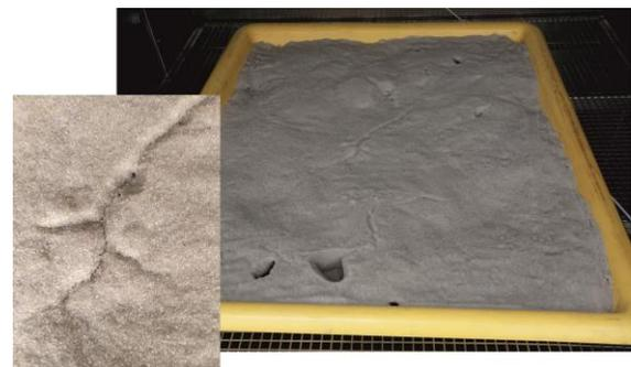
Fig.2. Experiment no 2. Wet sand with a layer of ice H<sub>2</sub>O underground.(amount of water used to produce ice: 2.5 l). This Fig.2 refers to Fig.3.
