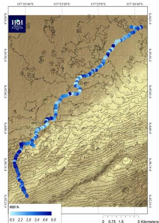
**Fig. 1.** Water content based on passive measurements of the DAN instrument. Each spot equal to 100m smoothing of the instrument data.
