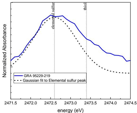
Figure 4: Gaussian fit to the elemental sulfur peak to calculate the residual due to the presence of thiol.
