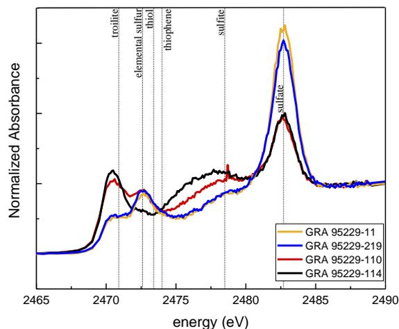
Figure 1: Typical  $\mu$ -XANES spectra in GRA 95229 showing the numerous peaks with different sulfur speciation. Each datapoint often shows multiple peaks.
