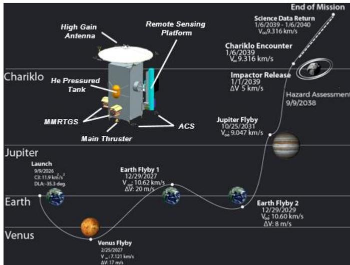
**Figure 1:** Concept of operations for a Centaur Reconnaissance mission with planetary encounter dates and delta velocity. Inset shows spacecraft configuration with labeled subsystems including: Multi-Mission Radioisotope Thermoelectric Generators (MMRTGs) and Attitude Control System (ACS).
