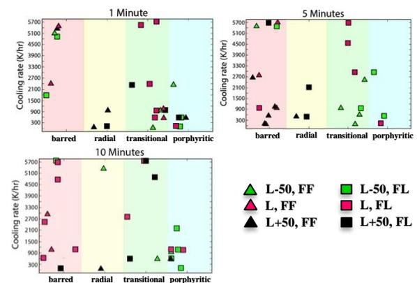
**Figure 1.** Cooling rates relative to texture type at different heating durations. *L*: liquidus = 1608 °C; *FF*: 63-90  $\mu\text{m}$  (olivine, albite, diopside); *FL*: 63-90  $\mu\text{m}$  (albite, diopside) and 212-250  $\mu\text{m}$  (olivine)
