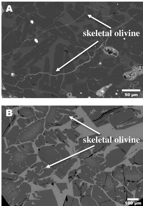
**Figure 2.** BSE images showing similar skeletal grains present in both meteoritic (A) and experimentally (B) produced textures using a 600 K/hr cooling rate.
