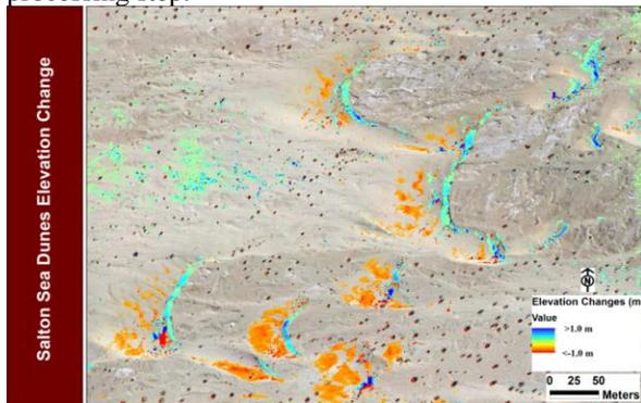
Figure 3. Elevation changes calculated from UAV data overlaid on the March 3<sup>rd</sup> orthophotomosaic. Values within  $\pm 20$  cm of 0 cm have been masked out due to uncertainties in the analysis. Red colors indicate erosion, while blue colors indicate deposition.
