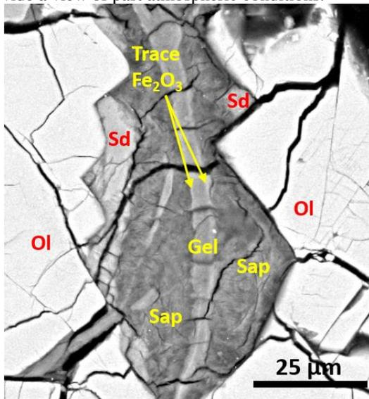
**Figure 1** - BSE image showing Lafayettes olivine(Ol)-hosted hydrothermal assemblage, consisting of siderite(Sd)-saponite(sap)-trace ferric oxide-amorphous smectitic gel.
