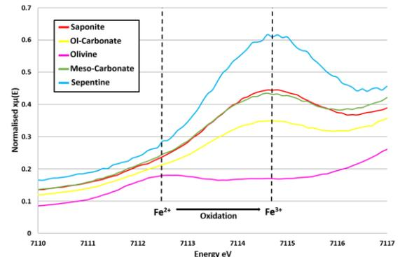
**Figure 4** - Fe-K XANES measurements were taken in order to gather information about the oxidation state of the Fe content. Pre-absorption edge features of Lafayette olivine (pink), ol-carbonate (yellow), ol-saponite (red), meso-carbonate (green) and meso-serpentine (blue) are shown.
