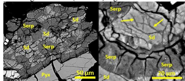
**Figure 2** - Left: BSE image of Lafayette mesostasis-hosted alteration assemblage, showing a texturally variable assemblage of siderite (Sd) precipitate partially replaced by a radially precipitated serpentine (Serp). Right: Close-up of mesostasis siderite being partially dissolved and replaced (arrow) by the adjacent serpentine.
