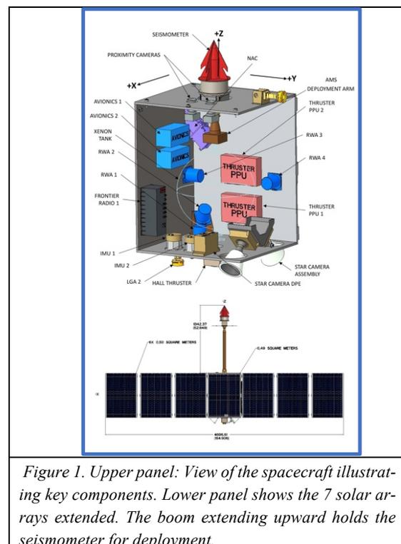
Figure 1. Upper panel: View of the spacecraft illustrating key components. Lower panel shows the 7 solar arrays extended. The boom extending upward holds the seismometer for deployment.
