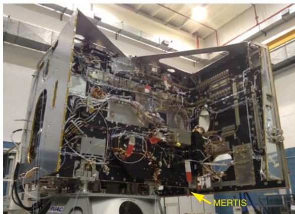
Figure 1: The BepiColombo MPO during early integration with the radiator panel facing to the right. The MERTIS planet baffle is visible at the bottom planet facing panel.
