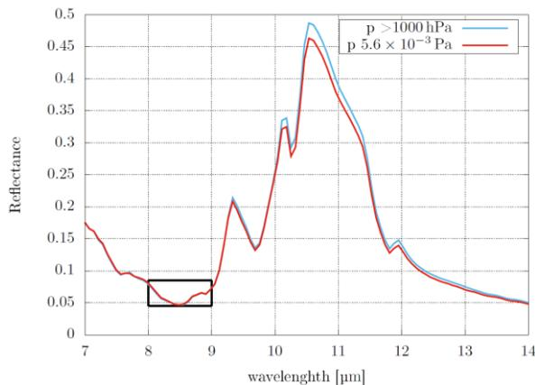
**Fig. 2:** Full olivine (63  $\mu\text{m}$  - 125  $\mu\text{m}$  fraction) reflectance spectra at room temperature and ambient pressure (blue line) and  $5.6 \cdot 10^{-3}$  Pa (red line). Box shows the CF displayed in Fig. 3.
