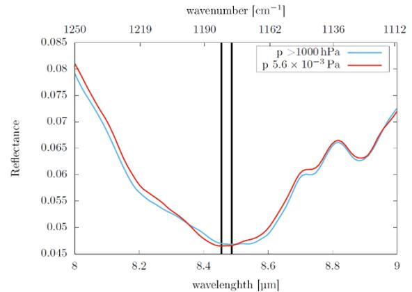
**Fig. 3:** Pressure-depended shift of the CF (marked with two black lines) of an olivine sample with grain size of 63 – 125  $\mu\text{m}$  at room temperature.
