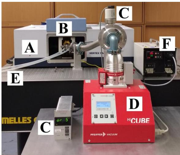
**Fig. 1:** The new setup in the IRIS lab: **A** Spectrometer with detector; **B** Praying Mantis with sample chamber; **C** Vacuum gauge head and corresponding controller; **D** Vacuum pump; **E** Flexible tubes for water cooling system, which cools the housing of the sample chamber; **F** Heat controller
