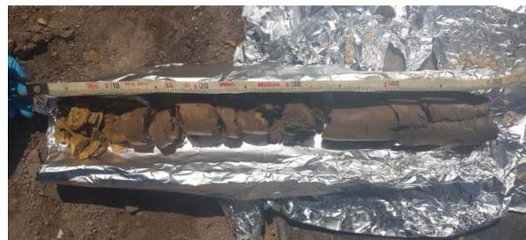
**Fig. 2.** Surficial section (30 cm) of the vibro-core collected as groundtruth of the Icebreaker drill.
