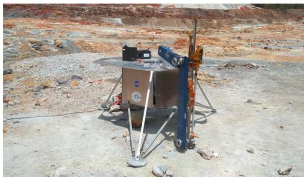
**Fig. 1.** Picture of the Icebreaker 1m-class planetary prototype drill, during the LMAP 2017 Rio Tinto field campaign.
