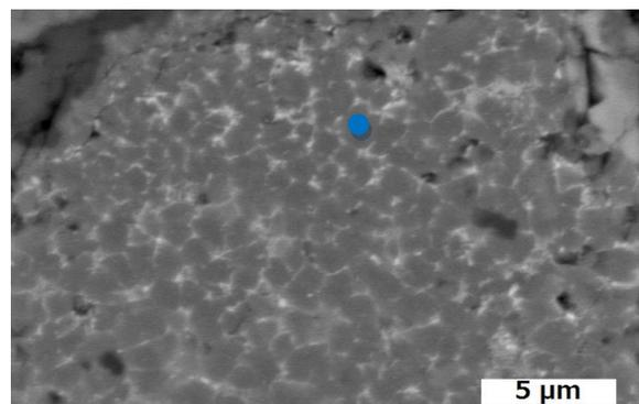
Fig. 5: BSE image of an enlarged portion of recrystallizing pyroxenes in a narrow shock vein.
