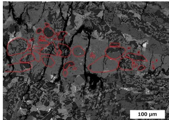
Fig. 4: BSE image of a relatively narrow shock vein which is composed of shock melted glass, relict mineral fragments (surrounded by red lines) and recrystallizing pyroxenes.
