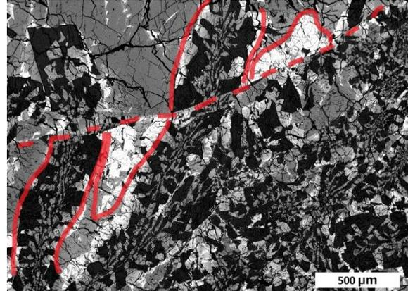
Fig. 3: BSE image of dendrites and pre-existing textures displaced by up to 1 mm as indicated by red lined areas. A shock vein (dotted line) cut them.
