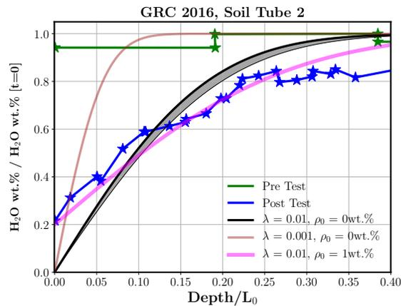
Figure 1: Final water distribution profile. Dark blue and green lines denote the “Post Test” and “Pre Test” experimental measurements, respectively. The grey region and magenta lines represent the model with parameters ( $\lambda = 0.01$ ,  $\rho_0 = 0$  wt.%) and ( $\lambda = 0.01$ ,  $\rho_0 = 1.00$  wt.%), respectively. The brown line shows the model presented at LEAG 2016, its parameters are ( $\lambda = 0.001$ ,  $\rho_0 = 0$  wt.%).
