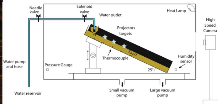
**Figure 1:** left: front view of a typical experimental run with the calibration board to the right, the water source at the back and a flow which has progressed past the three spotlights. Right: diagram of set up. Note the camera is actually positioned with a side-on view.
