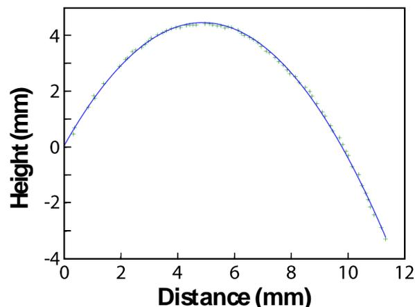
**Figure 3.** Example of a trajectory of a sand grain particle extracted from the high speed video. The green crosses are the points used for the ballistic fit (fitted curve in blue).
