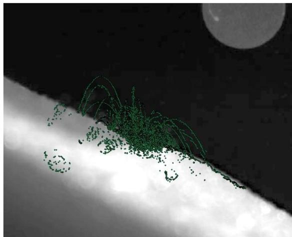
**Figure 2.** A screen capture of one of the high speed videos superposed with the grain trajectories extracted using *tractrac*. Circle in top-right is 7 mm across.
