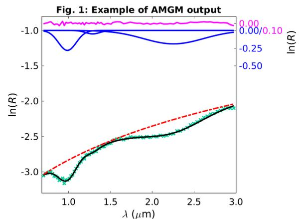
**Additional processing methods.** From AMGM, we obtain a set of spectral parameters (band widths, strengths, and positions, offset, slope, and curvature of a continuum) for every chosen spectrum within an area of interest. Typically, the studied area (e.g. fresh crater) contains information derived from tens to hundreds distinct spectral curves.
