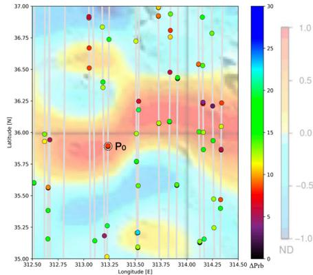
**Figure 2:** Locations presenting the characteristic features of two peaks echo patterns in Fig.1. The background image is a cross-correlation Bouguer gravity map referred from Chappaz et al. (2017)<sup>[5]</sup>.
