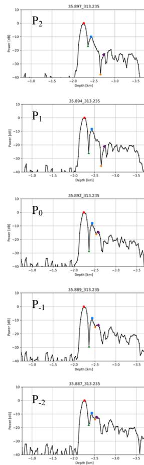
**Figure 3:** The LRS echo power versus the subsurface depth of a location  $P_0$  (35.892°N, 313.235°E) and its vicinity locations where echo features with two peaks was observed. The tendency that the echo powers of suggesting the existence of a subsurface layer or a wide cave.
