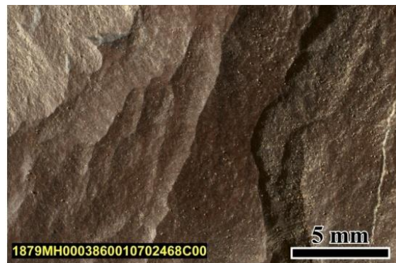
Fig. 5. MAHLI image of the Hexriver target (Sol 1879): a red mudstone from the VRR. DRT brushing did not leave any grooves suggesting that the target is very hard.
