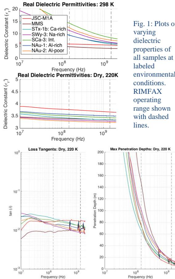
Fig. 1: Plots of varying dielectric properties of all samples at labeled environmental conditions. RIMFAX operating range shown with dashed lines.
