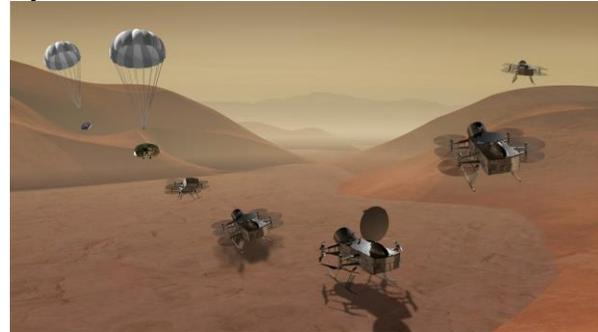
**Figure 4.** Artist conception of the rotorcraft operating on the surface of Titan. This vehicle would carry a suite of instrumentation for exploring the atmosphere and surface composition, and would include a germanium-based gamma-ray spectrometer.
