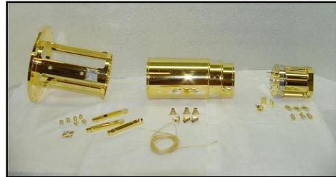
**Figure 1.** Infrared shielding for the germanium detector on NASA's MESSENGER mission to Mercury. Innovative IR shielding allows for cryogenic cooling in the harsh thermal environment.
