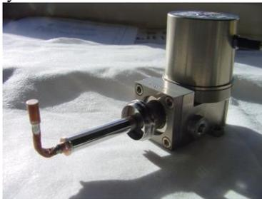
**Figure 3.** The Ricor k508 cryocooler has a mass of only 450 grams. It also has a very simple control circuit, eliminating a further 100 grams of controller board, as needed by other coolers.
