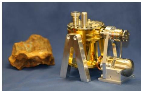
**Figure 2.** The prototype gamma-ray spectrometer for the Psyche mission. Also shown is an iron meteorite of material similar to that expected at (16) Psyche, used for testing and calibration.
