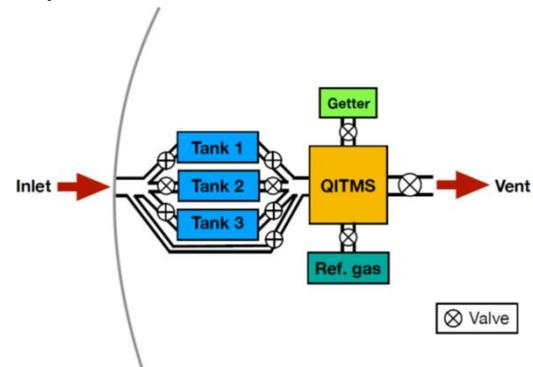
Figure 2: Schematic design of the QITMS and the different tanks in the probe. Using different valves, one can tailor the sampling strategy to best determine the concentration in noble gases in Venus' atmosphere.
