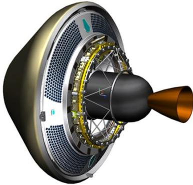
Figure 1: Artist concept of the Cupid's Arrow probe with the STAR 8 motor which would be ejected after VOI.
