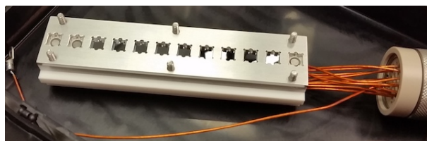
Fig. 5: Test fixture for whole-chip cathode activation. Twelve cathodes at a time can be loaded although only one at a time is activated.
