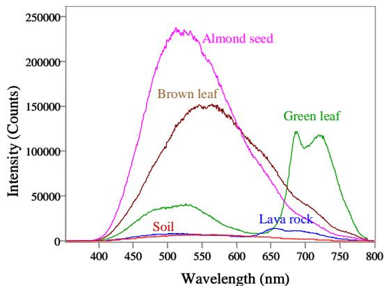
Fig. 4: Remote fluorescence spectra of various objects shown in Fig 2(a) with 355 nm excitation and 50 ns gate width.
