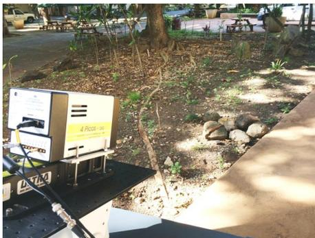
Fig. 1: Outdoor testing of Standoff Biofinder on a sunny day in Hawaii. The bio-images were collected from a collection of rocks as seen towards the right of the system at 3 m distance.
