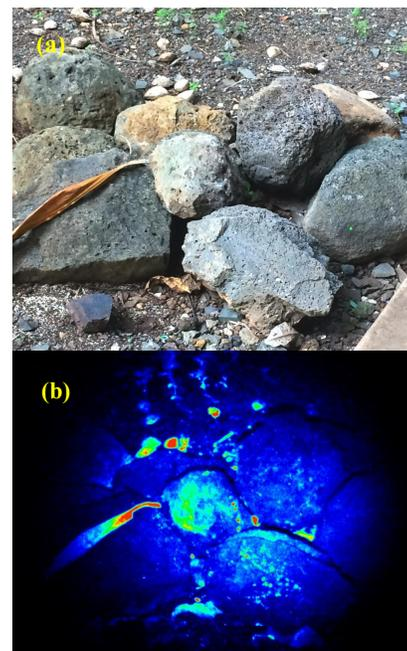
Fig. 2: (a) Picture of sample area captured using a regular color camera. (b) False-color bioimage of the target area using the Biofinder with 1 s integration time. The red areas indicate stronger fluorescence signal than the blue areas. Biological materials are detected on the lava rocks which appear to be free from bioactivity in the image (a).
