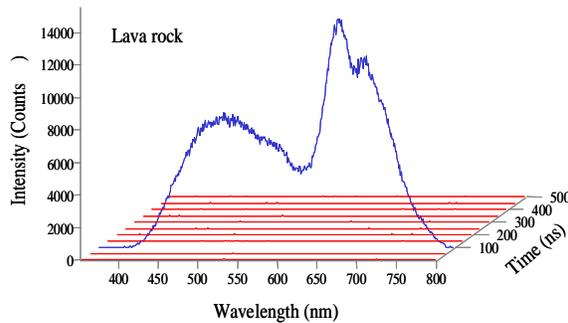
Fig. 3: Time resolved remote fluorescence spectra of lava rock with 355 nm excitation and 50 ns gate width separation. The fluorescence spectra predict presence of biological material on the rock.
