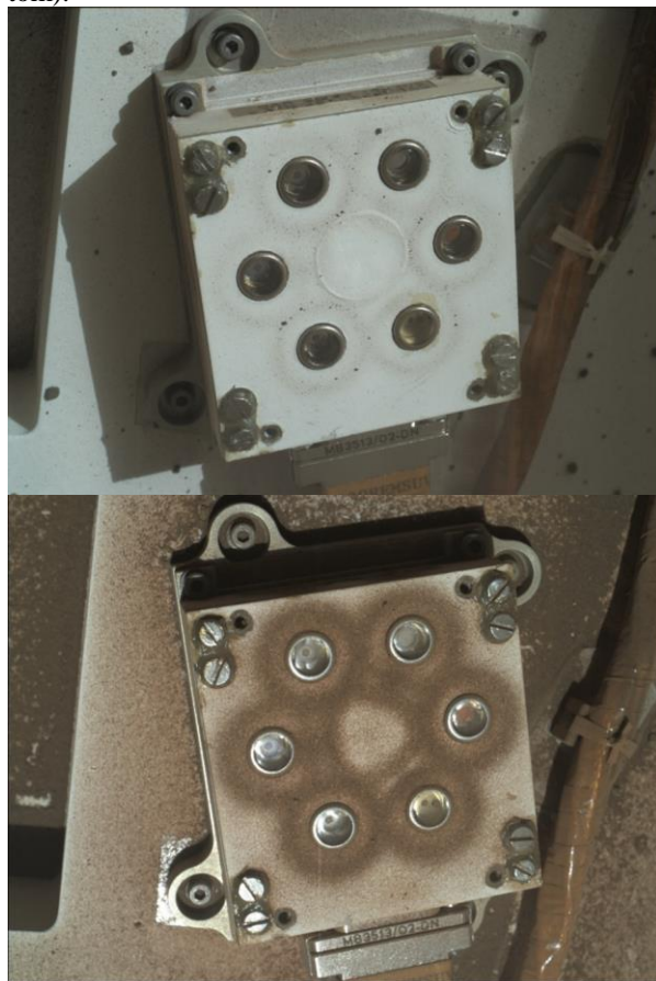
Figure 1. MAHLI images of the REMS UV Sensor on sols 36 (left) and 1314 (right). A significant amount of dust has been deposited on the sensor. The effect is particularly apparent around the circular magnets that
