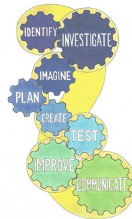
Figure 2: Figure of the Engineering Design Process utilized by middle school PLANETS units. The visual use of gears in this diagram helps youth to understand how each step is interconnected with and driven by others.
