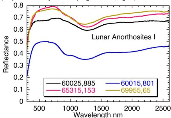
**Fig. 1.** Laboratory reflectance spectra of lunar anorthosite samples (RELAB BDR). All exhibit the diagnostic absorption near 1250 nm due to ferrous iron in plagioclase. 60015 also exhibits a weak feature (near 900 nm) mainly due to the presence of trace amounts of low-Ca pyroxene.
