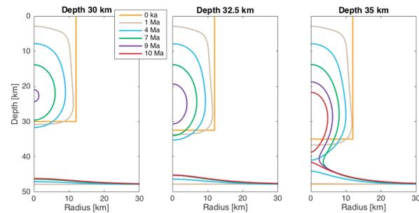
**Figure 2: Evolution of impact induced cryomagma chamber beneath Occator crater.** The solidus isotherm, bounding the magma chamber, is shown as function of time, see legend in left panel. Three panels show initial cryomagma chambers with increasing depth. The base of the crust below which deep brines are present is initially at 47.6 km.
