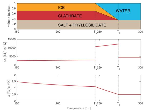
**Figure 1: Thermal model properties.** Top panel shows the volume fraction of phases as function of temperature. Middle panel shows the effective heat capacity of the multi-phase medium, including the latent heat term. Bottom panel shows the mean thermal conductivity of the multi-phase medium. Solidus temperature,  $T_s = 245^\circ\text{K}$ , is the eutectic temperature of relevant salt-ice mixtures [10]. The liquidus temperature,  $T_l = 273^\circ\text{K}$ , is the melting point of pure ice.
