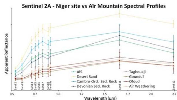
**Figure 2:** Spectral profile plots show the relative reflectance values of various rock types found in the Air region. Igneous plutons and their weathering products are grouped at the bottom with lower reflectance values while desert sand, sedimentary rocks, and the AIS show higher reflectance and display similarities between peaks of different wavelengths.
