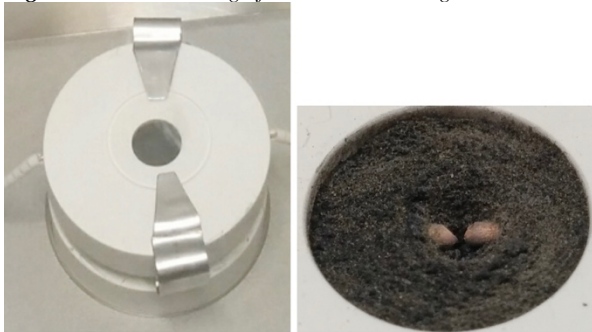
Figure 3. (Left) Ceramic sample holder in predecessor experiment configuration. (Right) 'Explosion crater' in JSC-1A sample produced by discharge between two electrodes buried in regolith from predecessor experiment [8].
